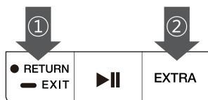
If your Samsung Smart Control is not paired to your TV, press and hold the buttons labelled ① and ② simultaneously for 3 seconds or more to pair the Samsung Smart Control to the TV.
