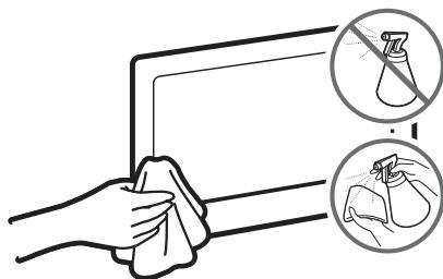
Do not spray water or any liquid directly onto the TV. Any liquid that goes into the product may cause a failure, fire, or electric shock.
