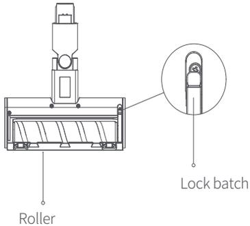
2. Rotate the end cover to the opening position and gently slide the roller from the suction head.
