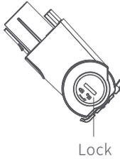
2. After removing the lock, remove the roller from the mite removal brush.
