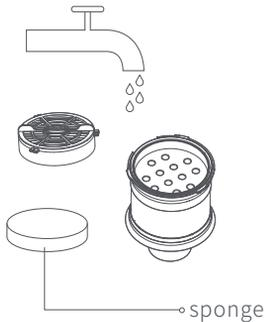
4. Dry the HEPA filter and steel filter components for at least 24 hours to ensure thorough drying, then put them back into the steel filter components
