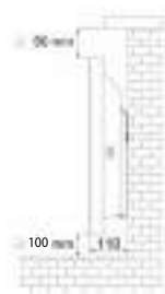
Figure 9. Dimensions of the convector after assembly
