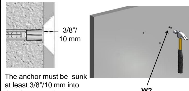
The anchor must be sunk at least 3/8" / 10 mm into the plaster coating
