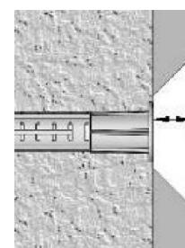
The anchor must be sunk at least 3/8" / 10 mm into the plaster coating
