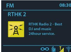
The first time you select FM radio mode, or if the station list is empty, the device will run auto scan
