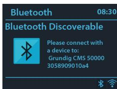
In Bluetooth mode, you can turn on the Bluetooth of your Bluetooth device. Press and hold »BTPAIR« to turns Bluetooth discoverable. From your Bluetooth device, search the HiFi System Grundig CMS 5000 to pairing. When it is waiting for pairing, there is a blinking Bluetooth icon at the bottom. If the pairing is successful, the Bluetooth icon becomes steady. Control the music playback from your Bluetooth device.
