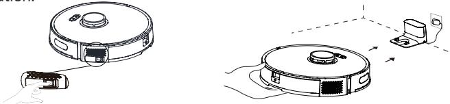
\* Place the machine on the charging dock and align it with the charging port. When the white indicator on the charging dock goes off, charging will begin.
