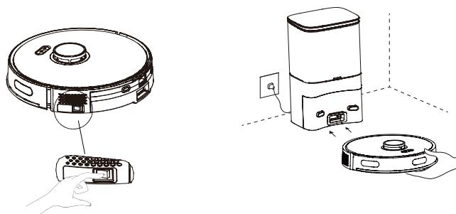
\* Manually place the vacuum cleaner on the dust collecting station and align it with the charging port. When the white indicator of the charging station flashes 3 times and then goes out, the charging will begin.
