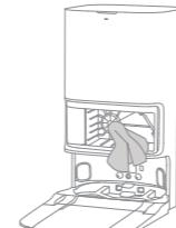
3. Install a new dust bag and reinstall the dust tank cover.
