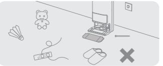
Before cleaning, please move away unstable, fragile, valuable or dangerous items, and clean up cables, cloths, toys, hard objects and sharp objects on the ground to avoid being entangled, scratched or knocked over by the robot and causing losses.
